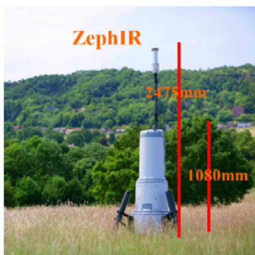
Photo 6: LIDARs for wind measurement – cost ~130.000 Euro
